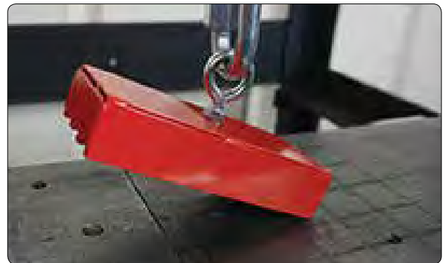
Breakaway force pull test.
