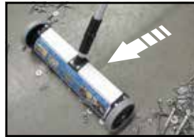
Roll over scattered ferrous metal to collect it...
